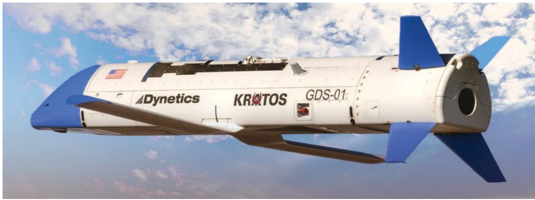
◀ A Dynetics-built X-61A Gremlin flew over Utah under a DARPA-sponsored program to test the feasibility of launching and recovering cruise-missile-sized drones from conventionally piloted aircraft. DARPA
