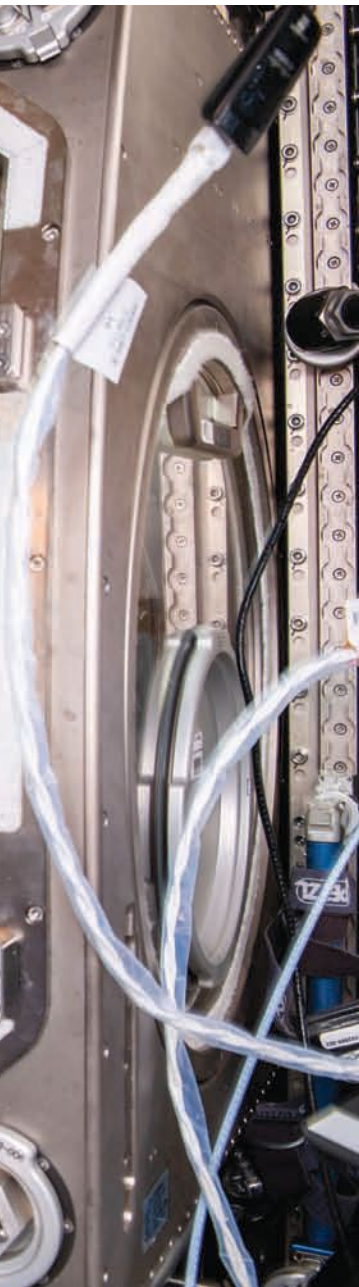
▲ This FOMS printer produced the company's first strands of ZBLAN aboard the ISS.
