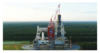
▲ The Space Launch System's core stage pathfinder is positioned in the B-2 Test Stand at NASA's Stennis Space Center in Mississippi. Crews practice handling skills with a pathfinder before working with the real core stage. NASA
