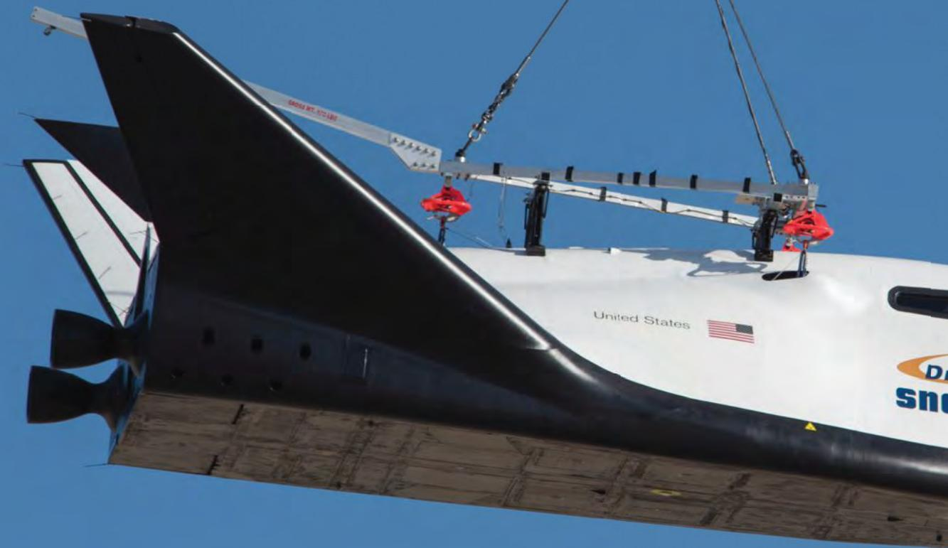
Sierra Nevada Corp.'s Dream Chaser test vehicle is hoisted by helicopter to its Nov. 11, 2017, free-flight test at Edwards Air Force Base, Calif.
