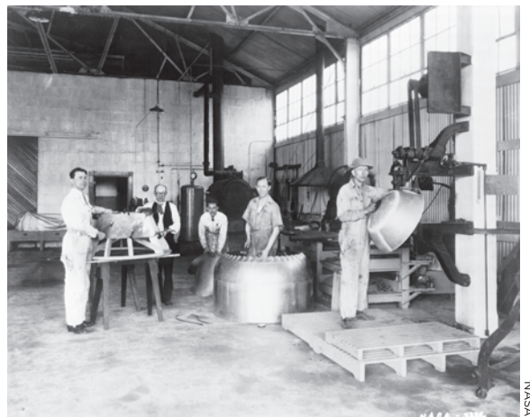
▲ Metal shop workers make engine cowlings, which smooth airflow over the engine and reduced drag.
