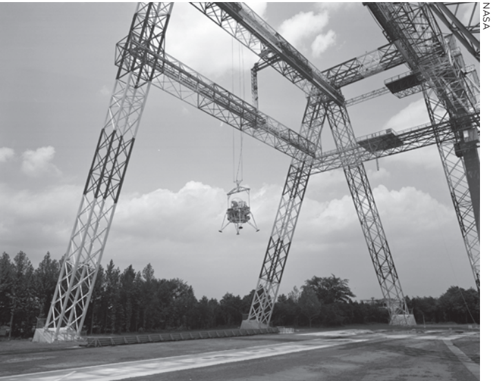
▲ Astronauts used Langley's gantry to practice the last 150 feet of the Apollo 11's descent to the moon's surface. Here it is in 1965.
