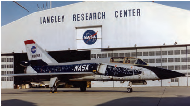
▲ The effects of many lightning strikes are visible on an F-106 used for storm research in 1982. The F-106 was another high-speed aircraft developed by Langley engineers and refined through extensive testing in the center's wind tunnels.
