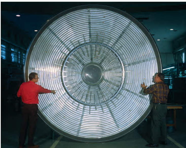
▲ NASA scientists at Langley examine the aeroshell that protected the Viking Lander 1 during its entry into the Martian atmosphere in 1976.
