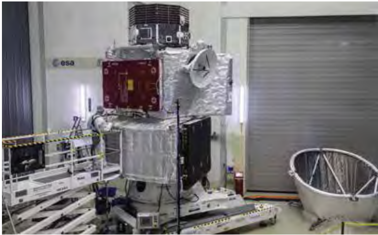
▲ The European Space Agency's BepiColombo spacecraft had its final launch readiness tests in July. The Mercury Magnetospheric Orbiter's Sunshield and Interface Structure (MOSIF) that will protect the MMO during the cruise to Mercury is sitting on the floor to the right.
