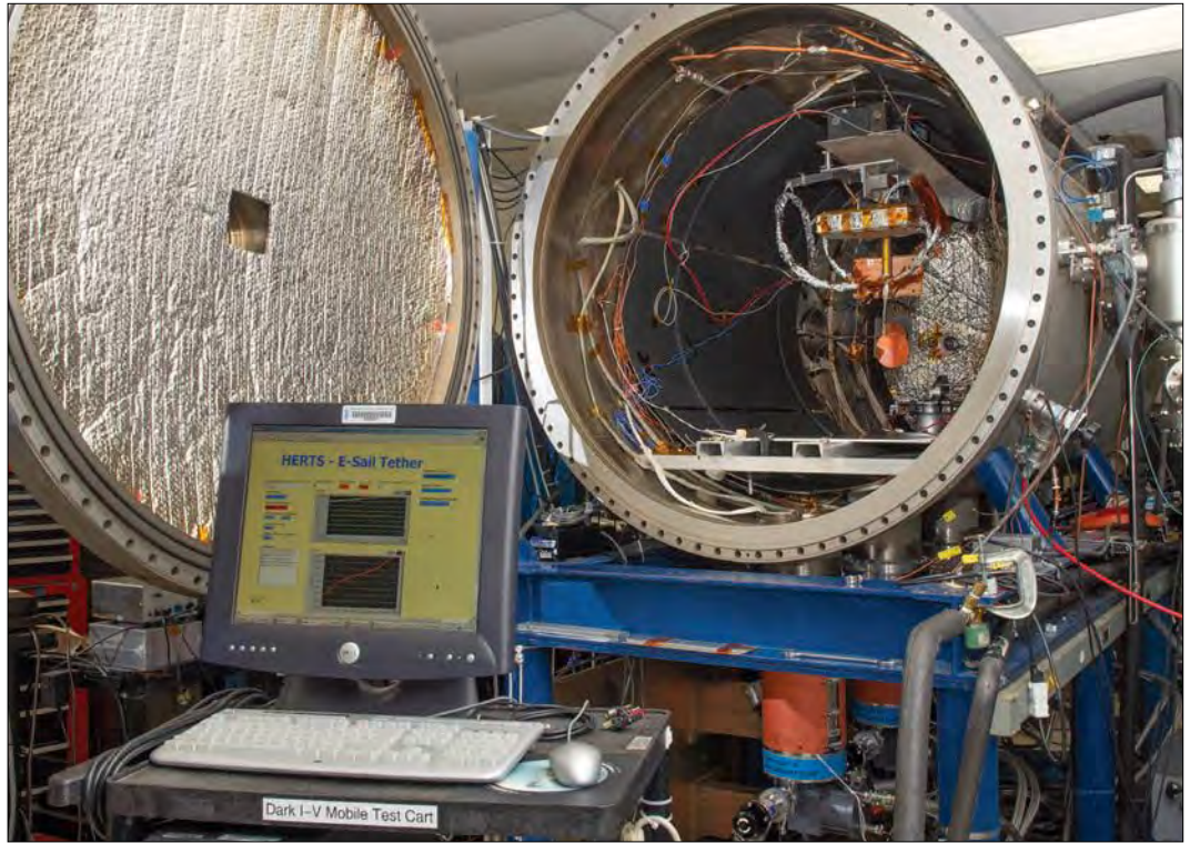
NASA is conducting tests inside a controlled plasma chamber, called the High Intensity Solar Environment Test system, to examine the rate of proton and electron collisions with a positively charged tether from a spacecraft’s electric sail.
