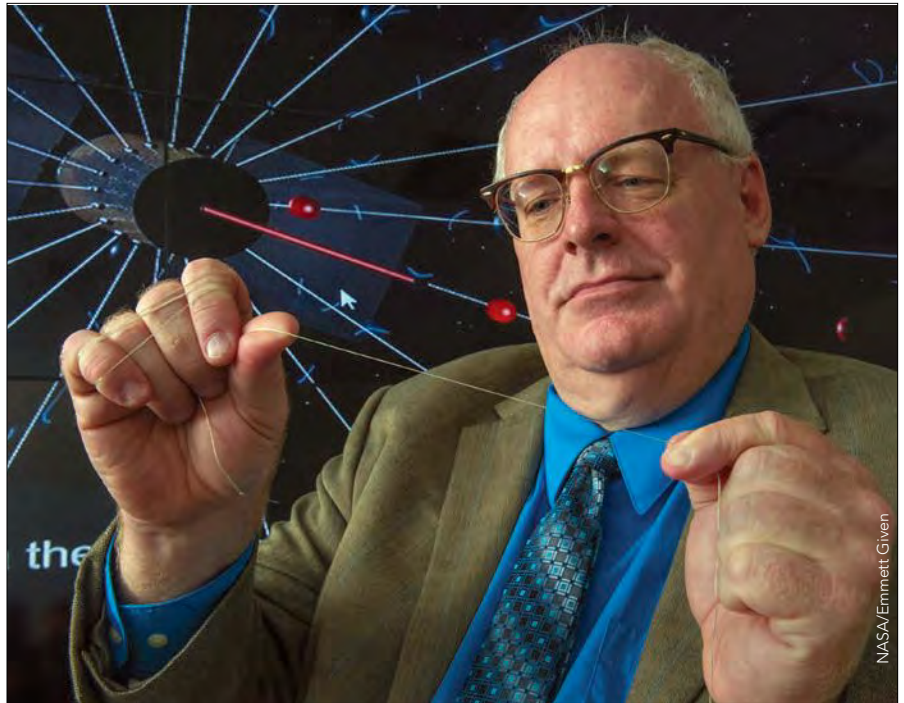
Bruce Wiegmann, principal investigator for NASA's Heliopause Electrostatic Rapid Transit System, holds a sample of Amberstrand composite string, one of the tether materials under investigation for use in a spacecraft propelled by electric sails. Behind him is an artist's concept for the electric sail.
