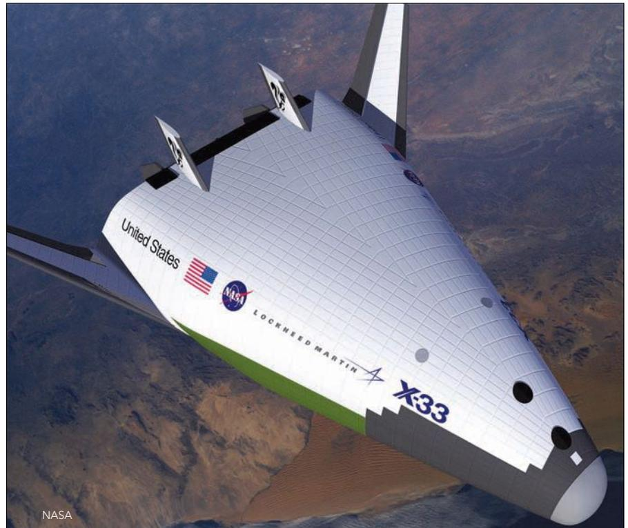
Lockheed Martin's X-33 was one of the failed attempts to build a single-stage-to-orbit space plane. NASA canceled it in 2001 in part because of its heavy weight, 92 percent of which was propellant.
