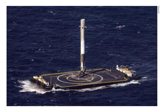
▲ In April, SpaceX for the first time landed the first stage of the Falcon 9 on a drone ship.
