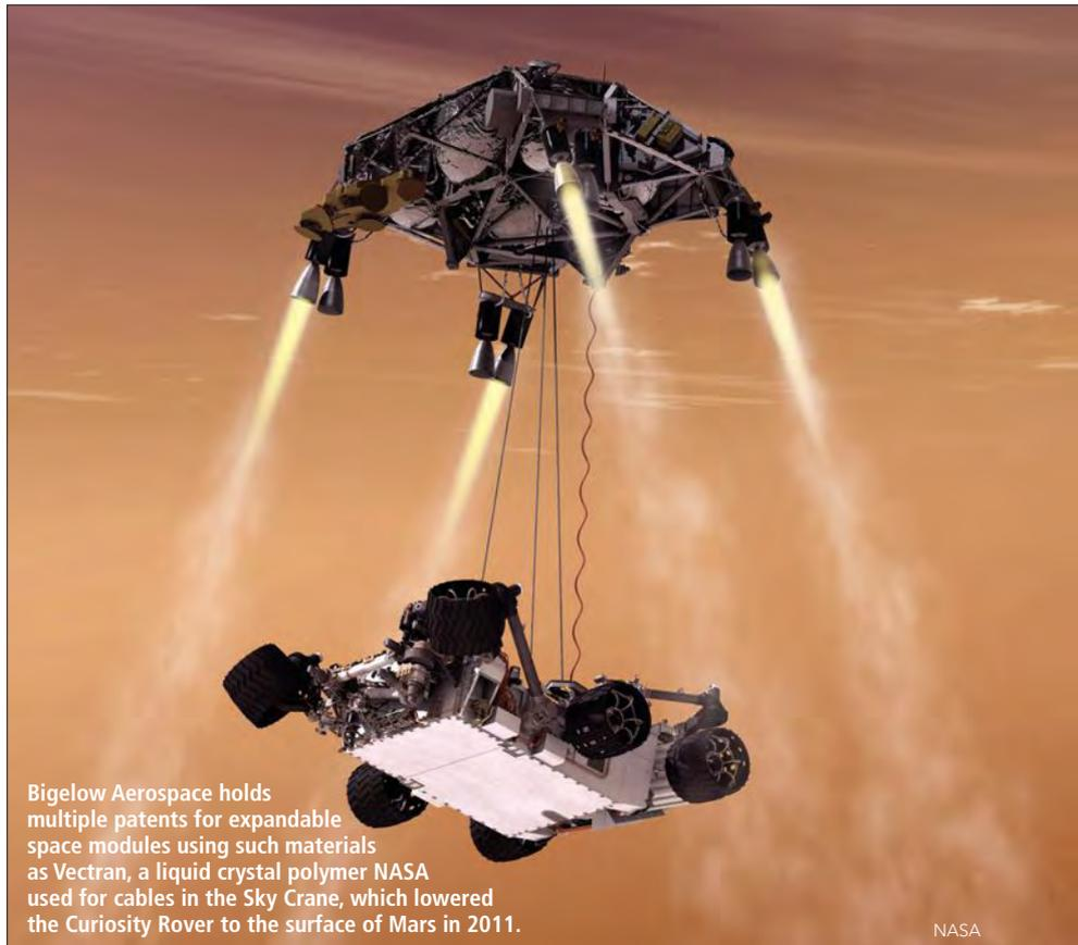
Bigelow Aerospace holds multiple patents for expandable space modules using such materials as Vectran, a liquid crystal polymer NASA used for cables in the Sky Crane, which lowered the Curiosity Rover to the surface of Mars in 2011.
