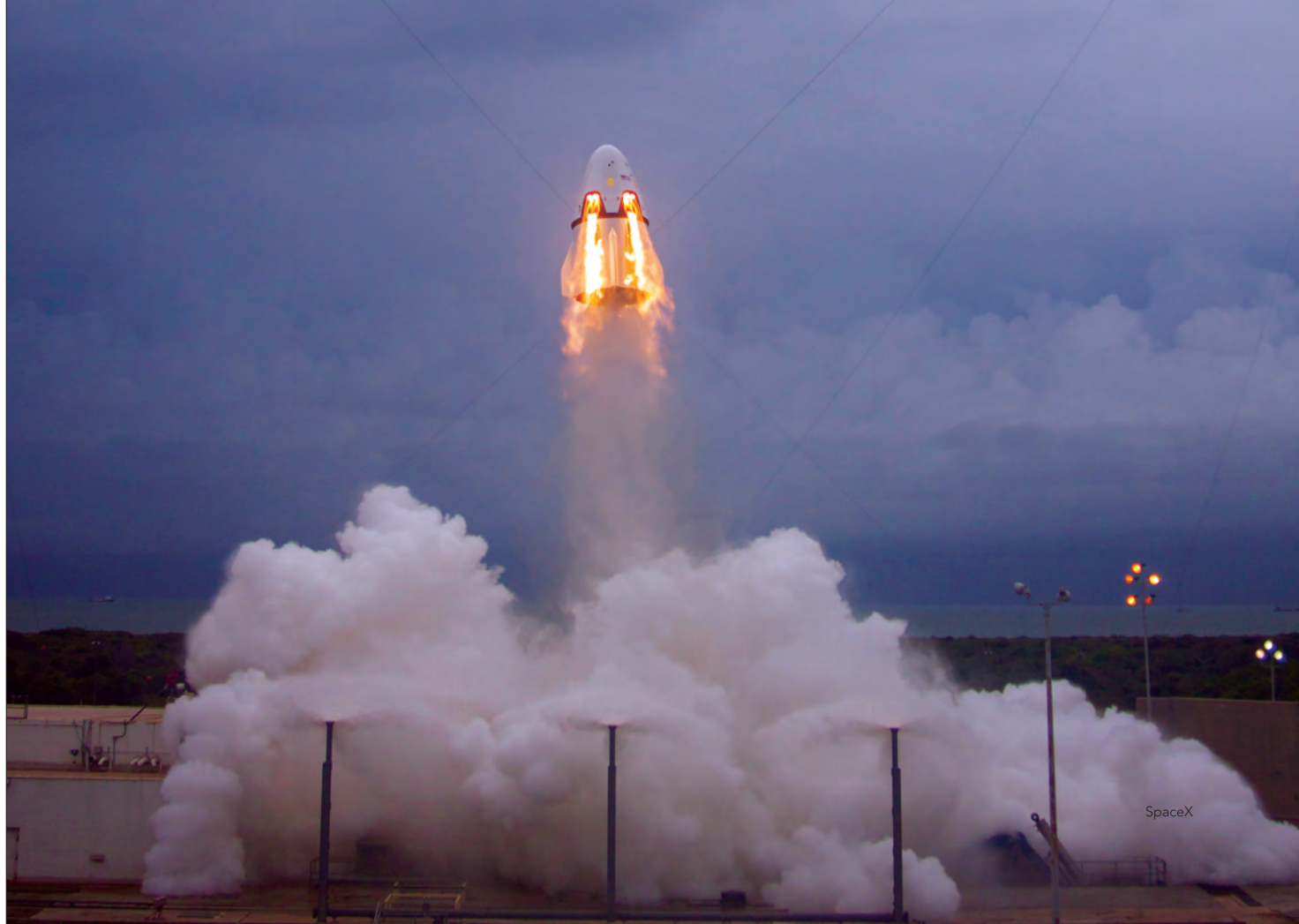
A SpaceX Crew Dragon lifts off during a pad-abort test in May. The unmanned test demonstrated how the capsule would save astronauts from a failing launch vehicle.
