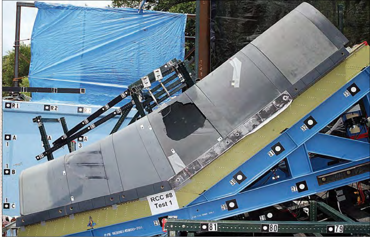
Fatal vulnerability: A chunk of foam like that on the shuttle's external tank pierced a section of reinforced-carbon-carbon material during testing at the Southwest Research Institute in Texas. Investigators concluded that foam fell from Columbia's tank during its 2003 ascent and damaged the orbiter's left wing, causing Columbia to burn up when the crew tried to return home after the mission.
