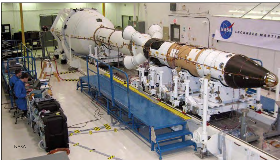
Technicians assess data collected during vibration tests on Orion's Launch Abort System. The inert, 16-meter-long assembly was tested in 2009 at the Orbital Sciences facility in Dulles, Virginia.
