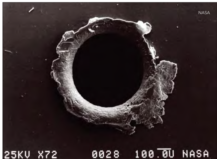
This impact mark was discovered on a component of the Solar Max scientific satellite after the space shuttle Challenger crew repaired the spacecraft in 1984. It is about the size of the period at the end of this sentence.
