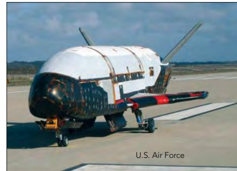
The U.S. Air Force's X-37B Orbital Test Vehicle taxis on the flightline in 2009 at Vandenberg Air Force Base, California. The secretive spaceplane is part of on-going efforts to develop reusable orbiters
