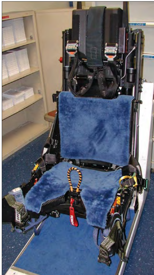
NASA has upgraded its T-38N jets with Martin Baker US16LN ejection seats to lessen danger to astronaut trainees. The seats can safely eject occupants even at zero altitude and zero airspeed.
