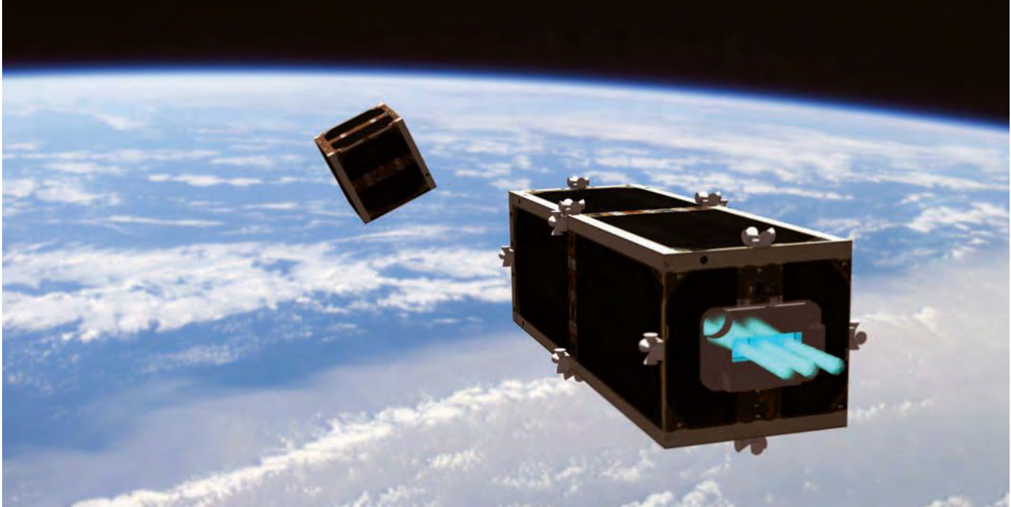
Photo illustration: The Swiss Space Center at École Polytechnique Fédérale de Lausanne CleanSpace One, a project to develop and build the first installment of a family of satellites specially designed to clean up space debris.
