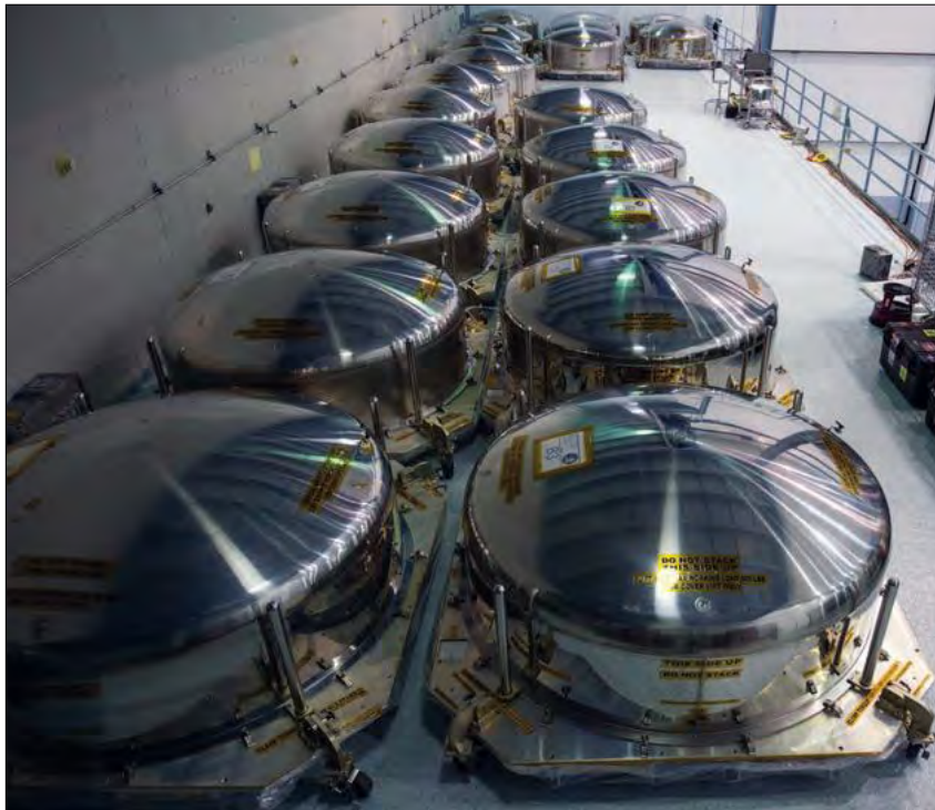
The mirrors of the James Webb Space Telescope shown in their shipping canisters at NASA's Goddard Space Flight Center in Maryland. Each of the 18 primary mirror segments is made of beryllium, which was selected mostly for its stability at cold temperatures.
