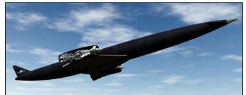
Reaction Engine's Skylon concept highlighting the SABRE engine.
