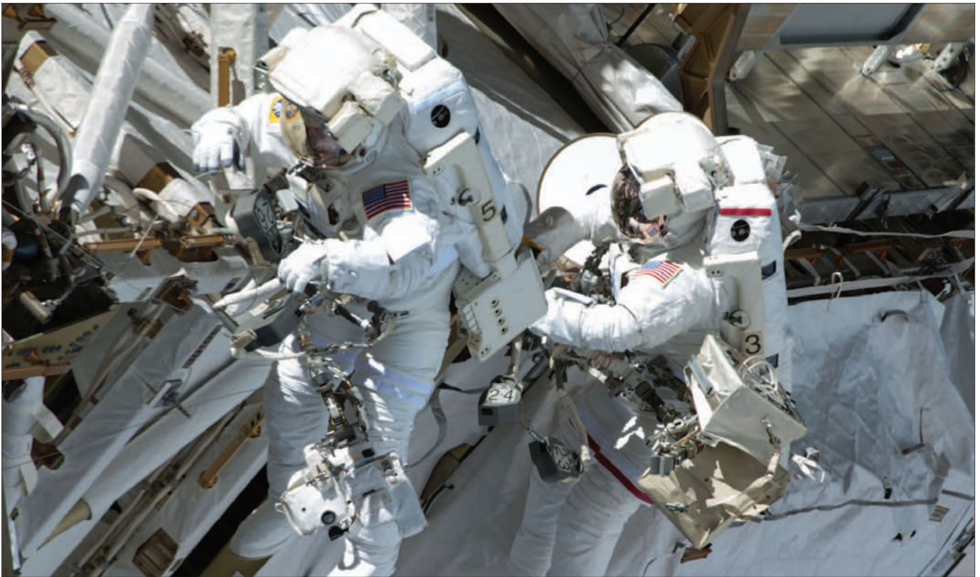
Expedition 35 flight engineers Chris Cassidy (right) and Tom Marshburn completed a space walk on May 11, 2013, to inspect and replace a pump controller box on the ISS's far port truss (P6) leaking ammonia coolant.
