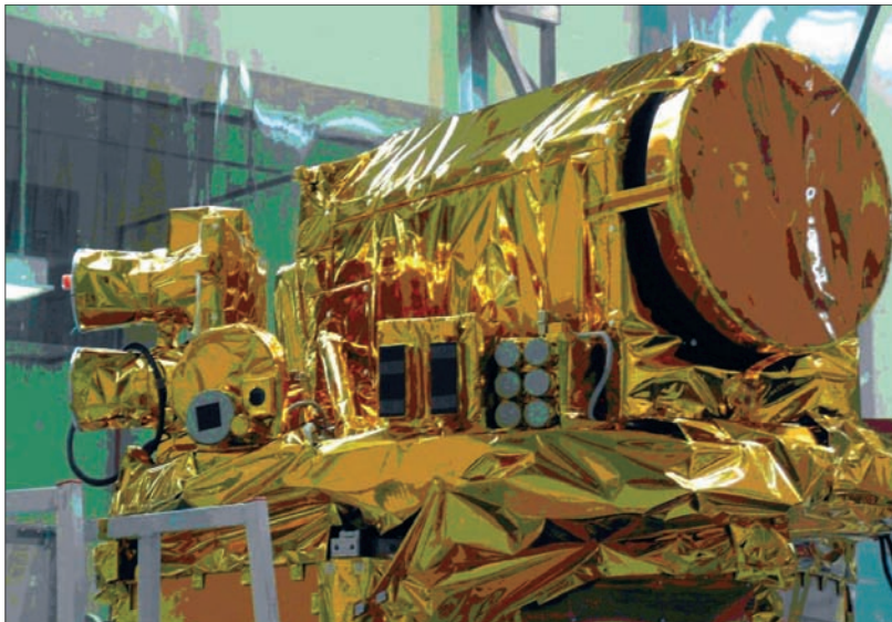
Formosat's large electrooptical imager can simultaneously capture four panchromatic, multispectrum images and then transmit the data to government agencies, private sector companies, and research organizations. Credit: Matra-Marconi/Taiwan National Space Program Office.
