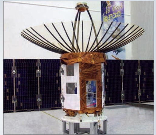
The Israeli-built TecSar day/night all-weather imaging radar satellite, which can also see through foliage, is being used by India to monitor Pakistan and China, especially the deployment of aircraft and armor. India launched a similar satellite for Israel. Credit: Israel Aircraft Industries.
