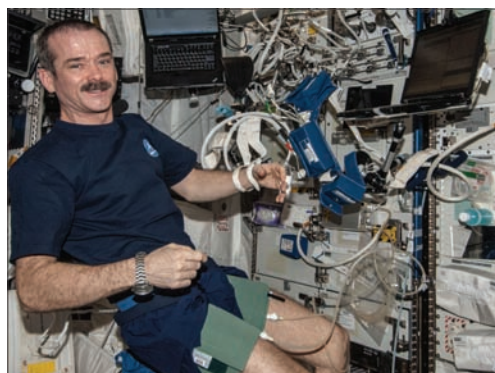
CSA commander Chris Hadfield uses the Human Research Facility pulmonary function system and the physiology module cardiolab leg/arm cuff system to conduct the first-ever session of this experiment. The test will help identify astronauts who could benefit from countermeasures before returning to Earth. This method has great potential for monitoring the health of the astronaut during future long-term spaceflights.
