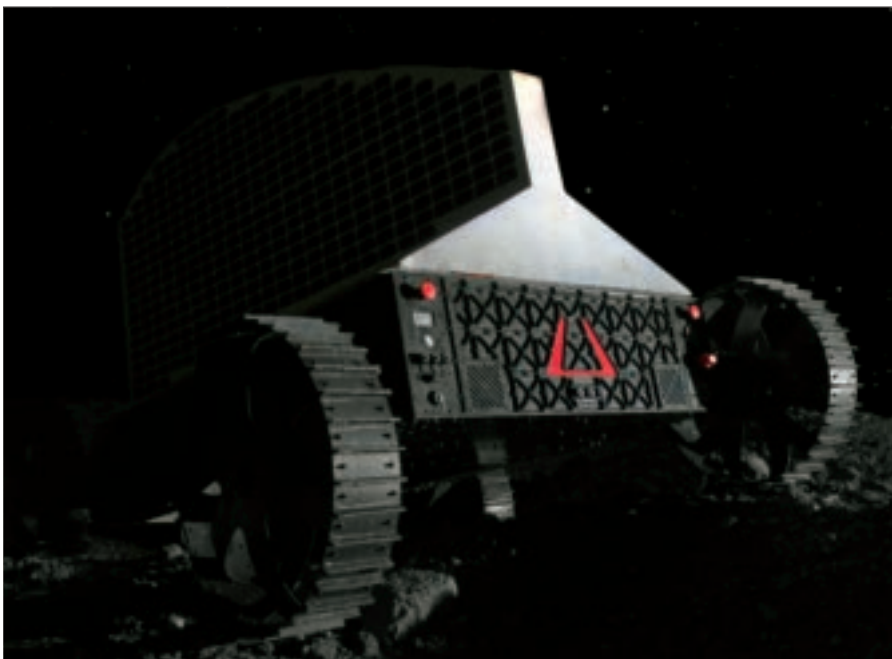
Commercially designed lunar ice prospectors, like this Polaris robotic rover from Astrobotic Technology, a spinoff of Carnegie Mellon University, can help NASA accelerate the search for valuable resources in Earth-Moon space. Courtesy Astrobotic Technology.
