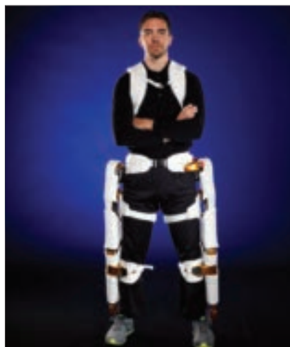
Project engineer Roger Rovekamp demonstrates the X1 robotic exoskeleton for resistive exercise, rehabilitation, and mobility augmentation in the Advanced Robotics Development Lab. Image credit: Robert Markowitz
