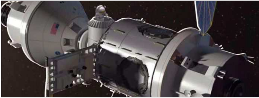
This concept for a translunar vehicle (TLV), capable of moving among the Earth-Moon Lagrange points and lunar orbit, would support periodic astronaut sorties beyond the lunar far side. Visiting Orion crews would engage in lunar scientific exploration, and perhaps examine and exploit a captured asteroid in high lunar orbit. Courtesy NASA.
