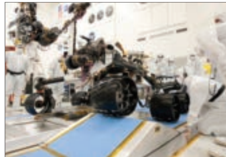
NASA’s Curiosity drives up a ramp during a test at JPL on September 10, 2010. The rover uses a rocker bogie suspension system to drive over uneven ground. Image Credit: NASA/JPL-Caltech.
