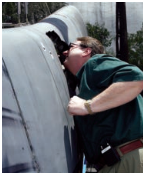
CAIB member Scott Hubbard inspects the damaged RCC panel 8 following a test. Credit: NASA/CAIB.
