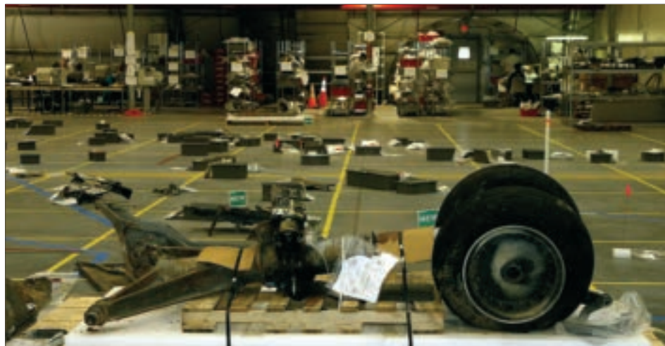
One of the larger pieces of recovered debris is Columbia's nose gear, shown here with tires still intact. Credit: NASA/CAIB.
