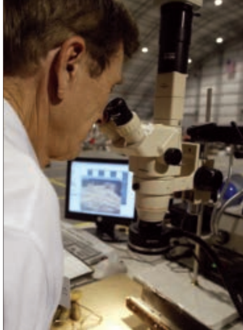
A reconstruction team member examines debris with a video-microscope, searching for clues to the events that led to Columbia’s breakup. Credit: NASA/CAIB.
