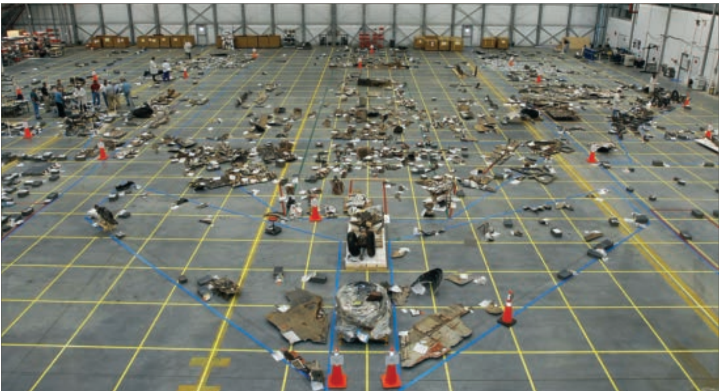
During search operations, this view of a KSC hangar shows a portion of the recovered pieces of Columbia debris. Credit: NASA Kennedy.
