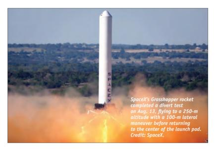
SpaceX also flew its **Grasshopper** experimental reusable rocket five times in 2013 to demonstrate the maneuverability of a re-usable launch vehicle. In August, the modified Falcon 9 performed a 100-m lateral maneuver, reached an altitude of 250 m, and safely returned to the center of the launch pad, making it the first test flight to include a lateral component. Grasshoppper has reached an altitude of 744 m in the flights from the company's Rocket Development Facility in McGregor, Texas.
