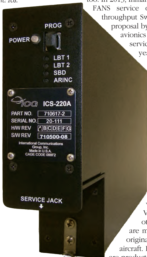
ICG's NxtLink ICS-220A Iridium Communications System combines data modem and dual voice/data transceivers. Credit: ICG.
