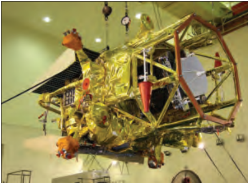
The loss of Phobos Grunt was originally blamed on the use of "non-space-qualified" microchips.
