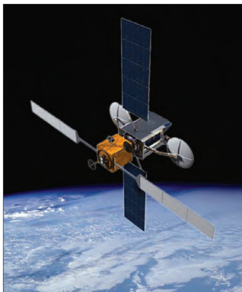
ViviSat uses ATK's Mission Extension Vehicle to safely connect to an orbiting satellite to provide attitude and propulsion capabilities without disrupting the client satellite's operation.
