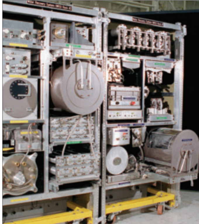
The WRS provides clean water through the reclamation of waste waters.
