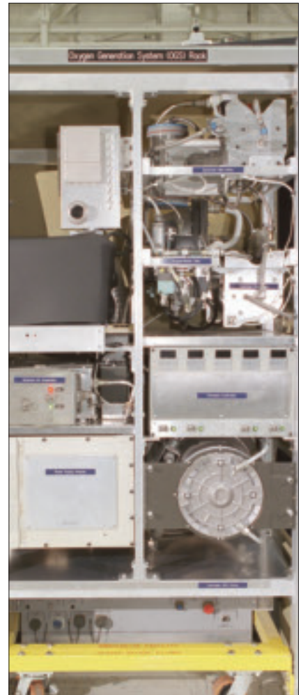
An oxygen generation system uses electricity from station solar panels to generate breathable oxygen through electrolysis.
