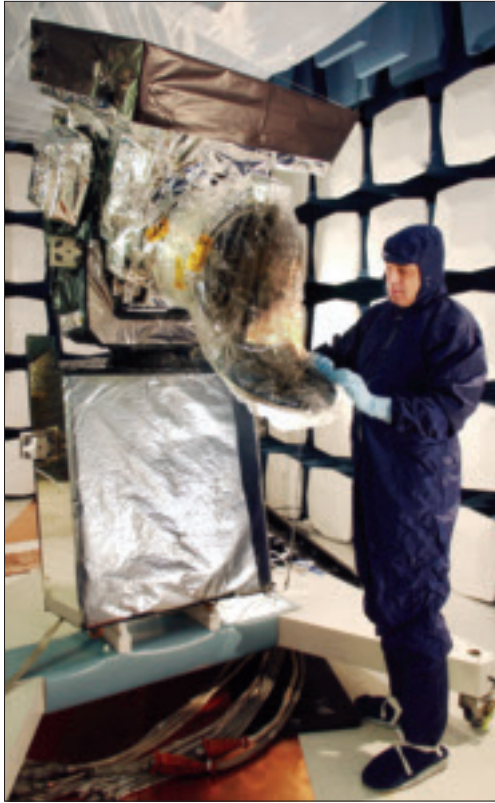
The second HEO payload, a critical element of SBIRS, undergoes final inspection prior to delivery.
