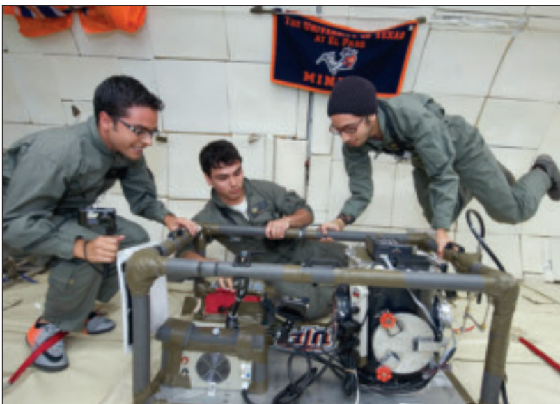
Students at the University of Texas at El Paso investigated self-sustained combustion of JSC-1A lunar regolith simulant mixed with magnesium on a reduced gravity aircraft flight.
