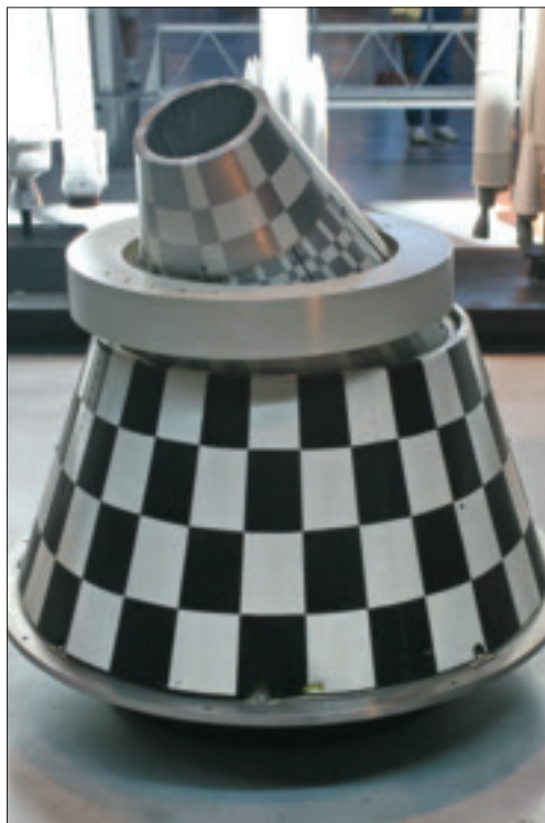
This sensor infrared alarm system was part of the 1950s MiDAS program.
