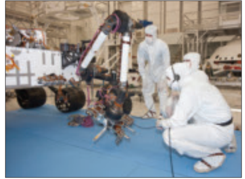
Curiosity’s 7.5-ft robotic arm, which will use a percussion device to break rock into powder, is much stronger than the 3-ft MER arms.
