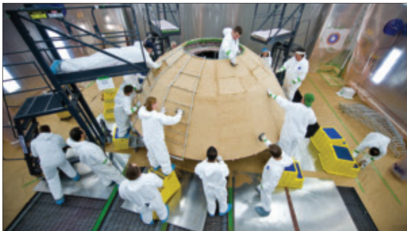
The aeroshell is a blunt-nosed cone that will encapsulate and protect Curiosity during its deep space cruise to Mars, and from the intense heat and friction that will be generated as the system descends through the Martian atmosphere. Credit: Adam Mattivi, courtesy Lockheed Martin.
