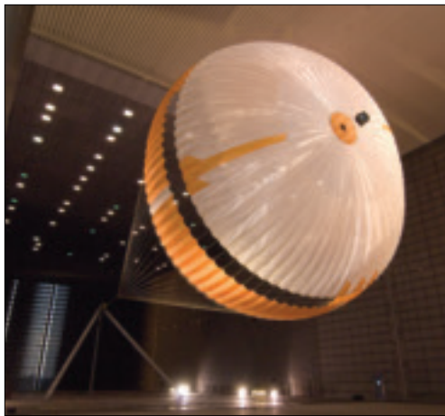
An MSL parachute test is conducted at the Ames/NFAC 80x120 wind tunnel. Credit: T. Wynne.
