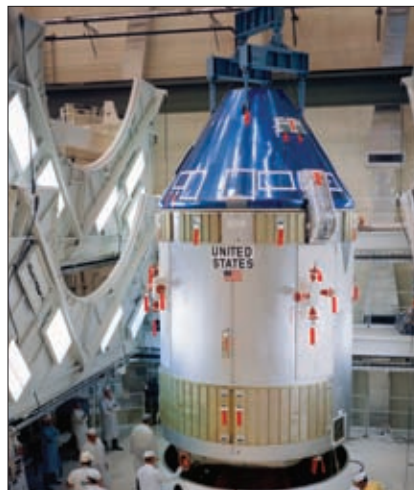
Technicians move the Apollo 7 CSM into position for mating with the spacecraft LM adapter.
