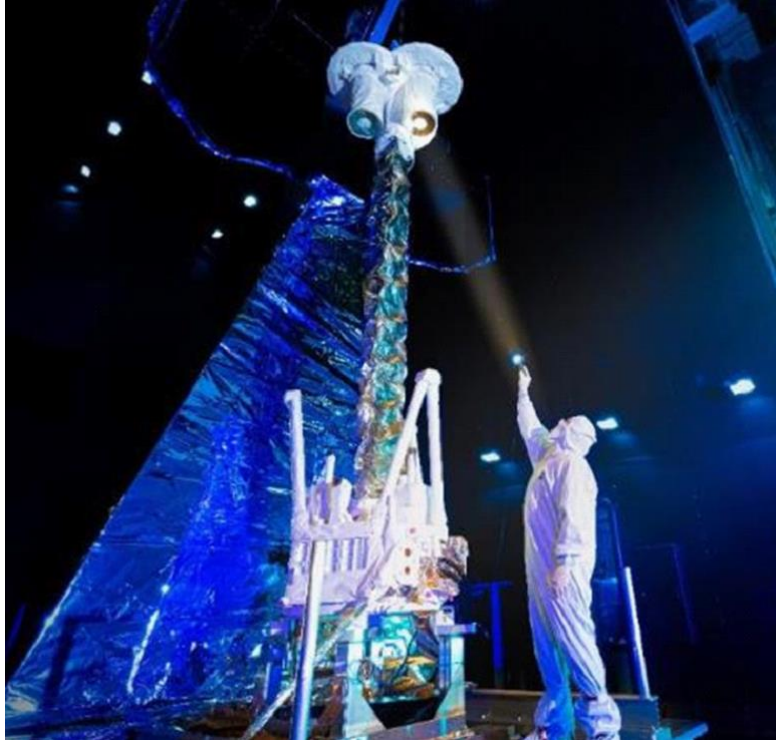
Figure 3: Photograph of IXPE with the boom deployed in a thermal vacuum chamber (TVAC) during Observatory environmental testing. When deployed, IXPE is 5.2 m from the bottom of the Spacecraft structure to the top of the payload and is 1.1 m in diameter. The solar panels, removed for TVAC, span 2.7 m when deployed. Photo courtesy of Ball Aerospace.
