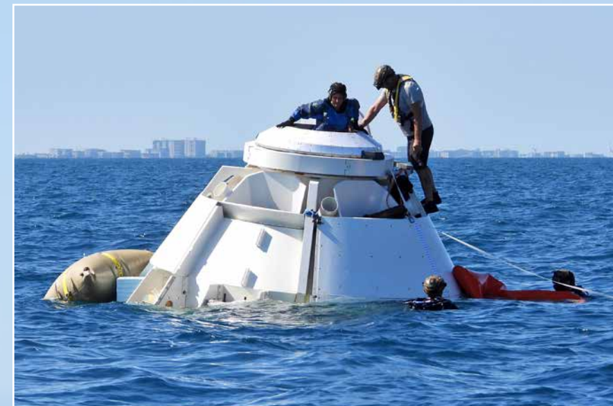
NASA astronaut Suni Williams, at left, rehearses the steps she would take to exit Boeing's CST-100 Starliner spacecraft without assistance in the unlikely event of an emergency result in a splashdown on April 27, 2019 off the coast of Cape Canaveral near NASA's Kennedy Space Center. Photo credit: NASA/Michael Downs
