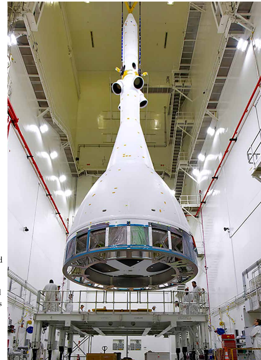
Above: A test version of the Orion crew module was integrated with the Launch Abort System on May 18, 2019. It was then lifted by crane for transfer to a KAMAG transporter. Photo credit: NASA/Glenn Benson
