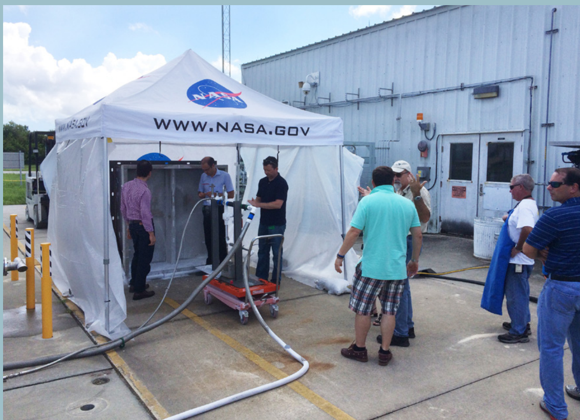
Members of Kennedy Space Center's Cryo Test Lab team set up the cold vapor test in which a newly developed nozzle created a wall of mist against a test panel loaded with sensors. Photo credit: NASA
