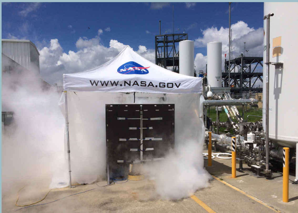
The test panel is shrouded in mist during the cold vapor test, which was designed to help establish a new test standard. Photo credit: NASA
