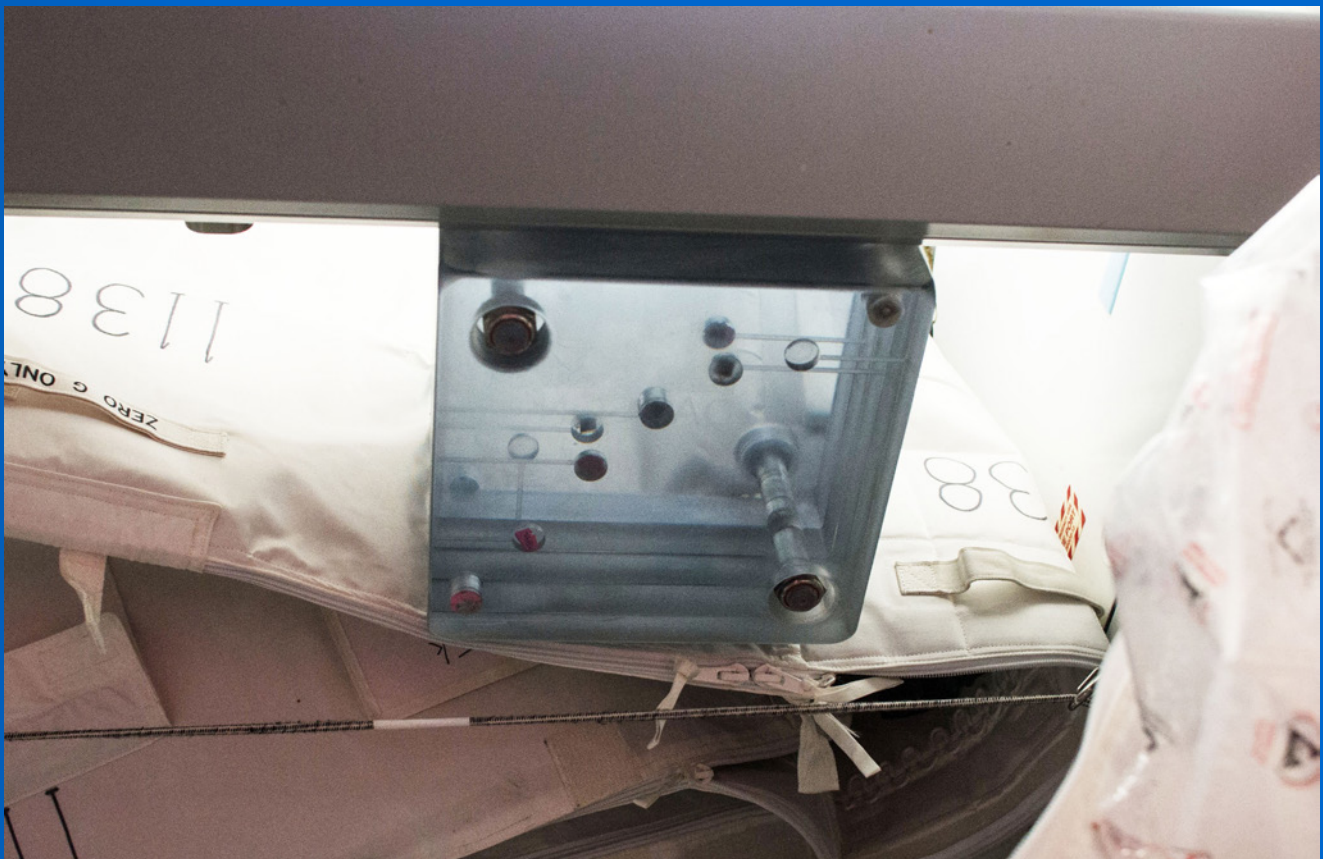
A sensor designed to detect radiation damage and materials fatigue now is at work aboard the International Space Station. The Detector for the Analysis of Solar Neutrons, or DANSON, was developed at the University of Nebraska. It was installed by NASA astronaut Shane Kimbrough shortly after its arrival aboard the Cygnus spacecraft. Such a device could generate electricity similar to a solar cell, but from neutrons instead of photons, to power NASA's future deep space probes. Photo credit: NASA
