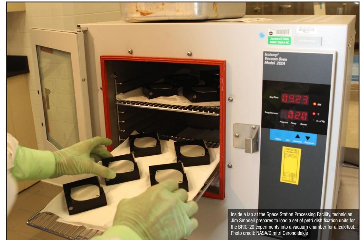
Inside a lab at the Space Station Processing Facility, technician Jim Smodell prepares to load a set of petri dish fixation units for the BRIC-20 experiments into a vacuum chamber for a leak test. Photo credit: NASA/Dimitri Gerondidakis
