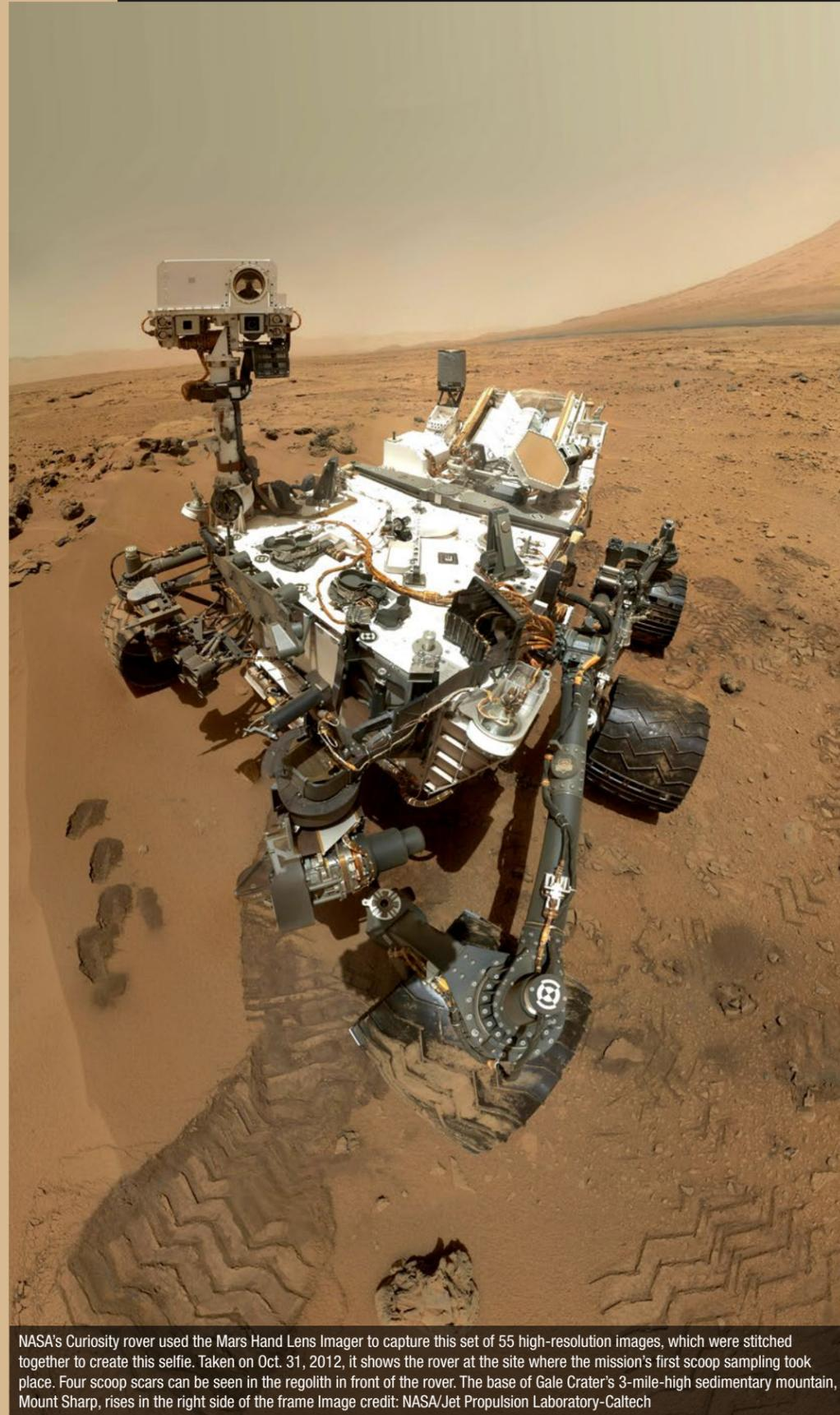
NASA's Curiosity rover used the Mars Hand Lens Imager to capture this set of 55 high-resolution images, which were stitched together to create this selfie. Taken on Oct. 31, 2012, it shows the rover at the site where the mission's first scoop sampling took place. Four scoop scars can be seen in the regolith in front of the rover. The base of Gale Crater's 3-mile-high sedimentary mountain, Mount Sharp, rises in the right side of the frame. Image credit: NASA/Jet Propulsion Laboratory-Caltech
