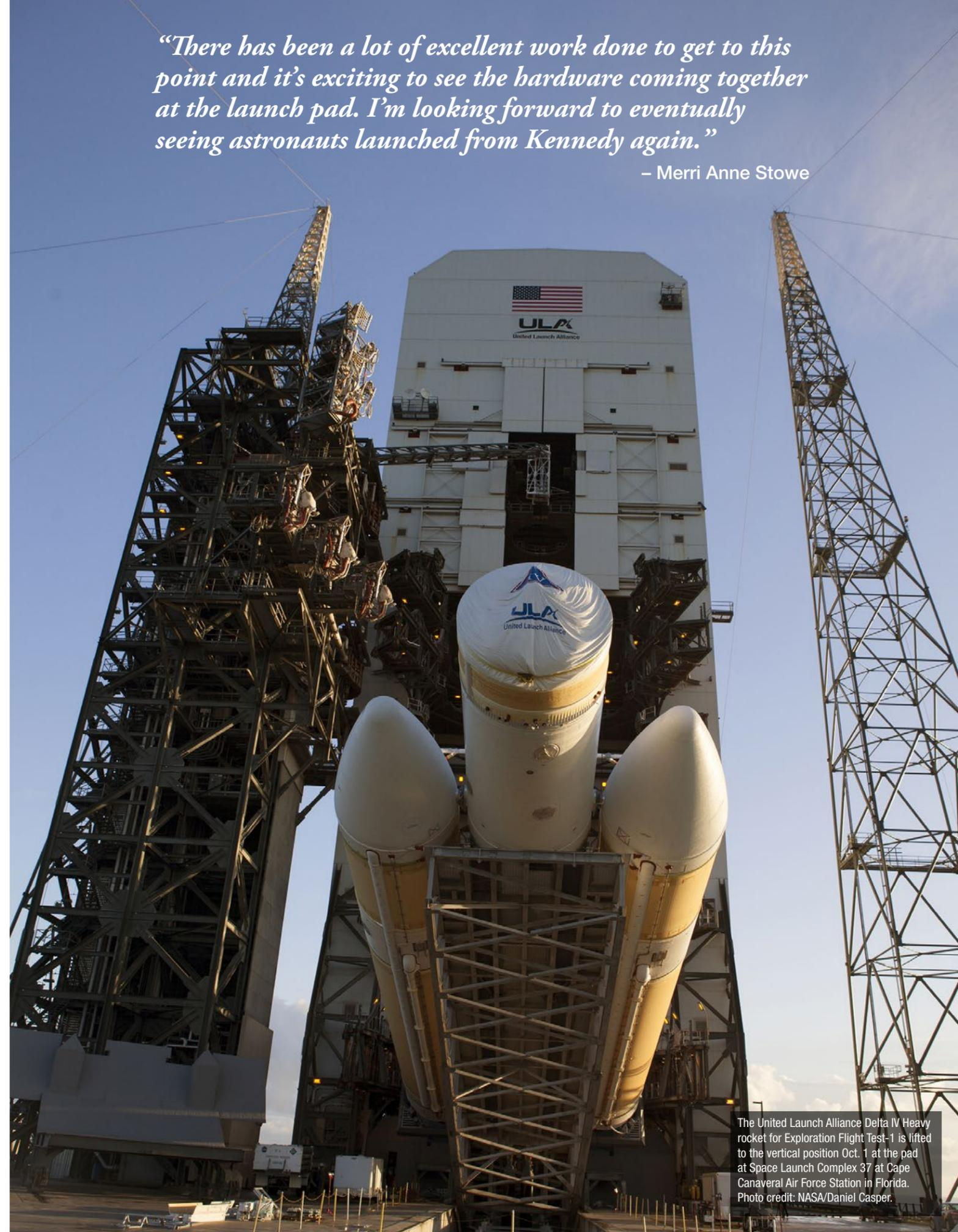
The United Launch Alliance Delta IV Heavy rocket for Exploration Flight Test-1 is lifted to the vertical position Oct. 1 at the pad at Space Launch Complex 37 at Cape Canaveral Air Force Station in Florida. Photo credit: NASA/Daniel Casper.
