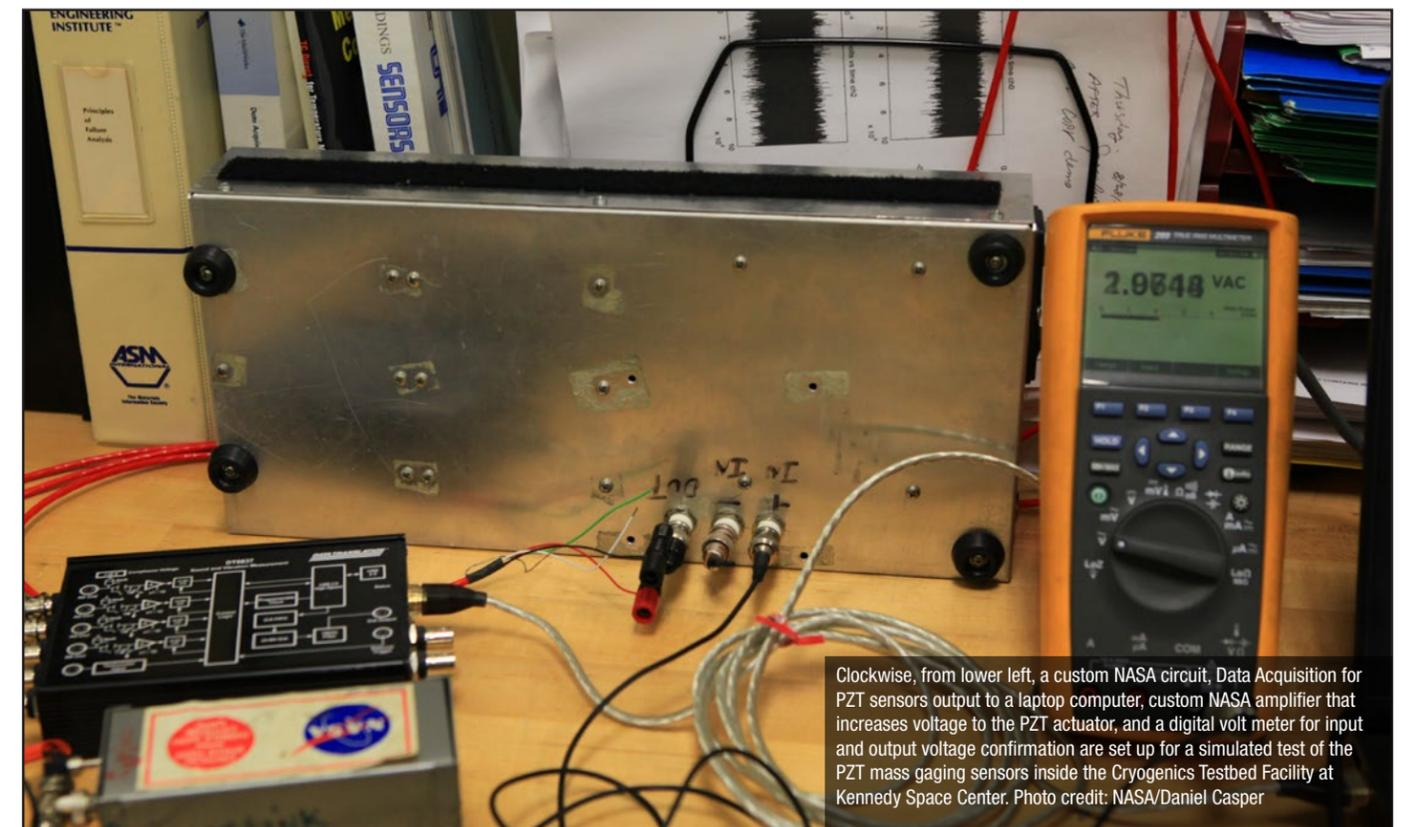
Clockwise, from lower left, a custom NASA circuit, Data Acquisition for PZT sensors output to a laptop computer, custom NASA amplifier that increases voltage to the PZT actuator, and a digital volt meter for input and output voltage confirmation are set up for a simulated test of the PZT mass gaging sensors inside the Cryogenics Testbed Facility at Kennedy Space Center. Photo credit: NASA/Daniel Casper
