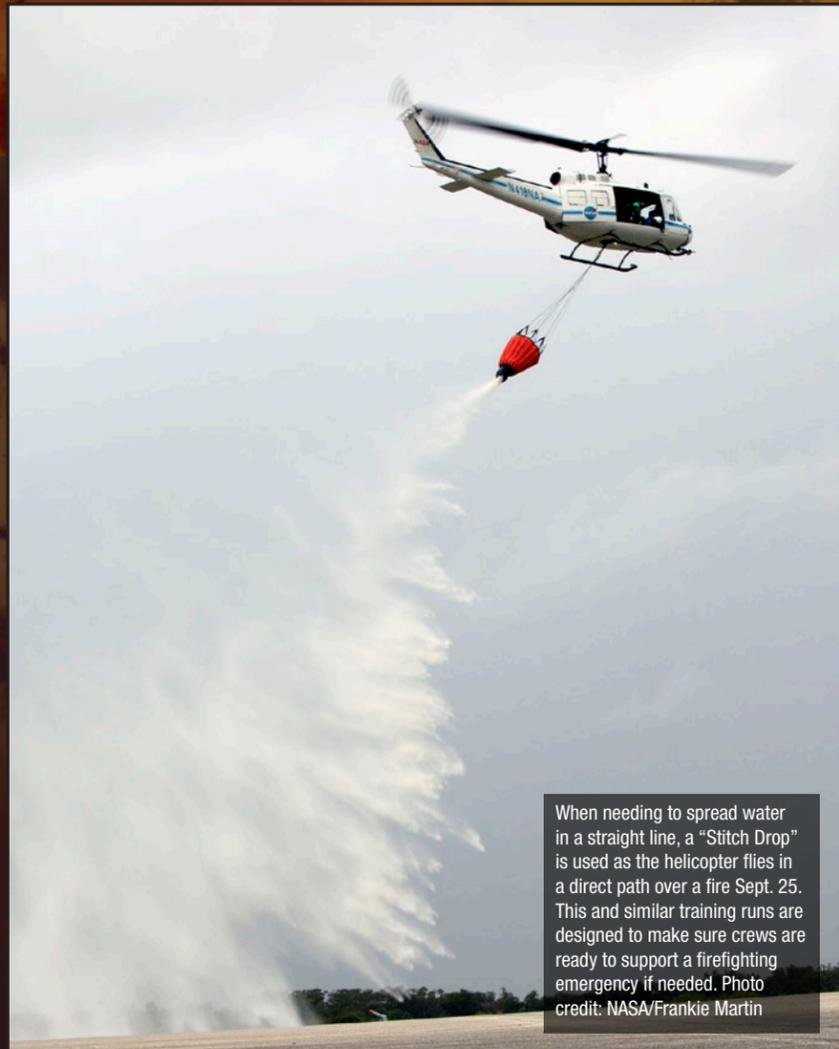
When needing to spread water in a straight line, a “Stitch Drop” is used as the helicopter flies in a direct path over a fire Sept. 25. This and similar training runs are designed to make sure crews are ready to support a firefighting emergency if needed. Photo credit: NASA/Frankie Martin
