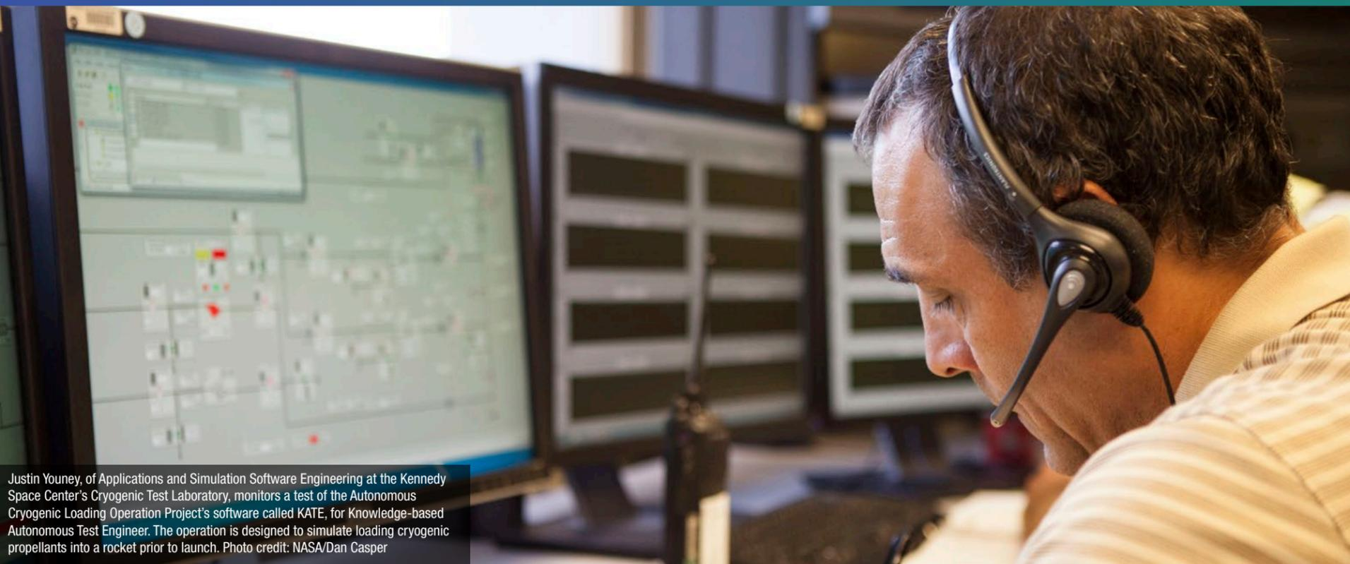
Justin Youney, of Applications and Simulation Software Engineering at the Kennedy Space Center's Cryogenic Test Laboratory, monitors a test of the Autonomous Cryogenic Loading Operation Project's software called KATE, for Knowledge-based Autonomous Test Engineer. The operation is designed to simulate loading cryogenic propellants into a rocket prior to launch. Photo credit: NASA/Dan Casper
