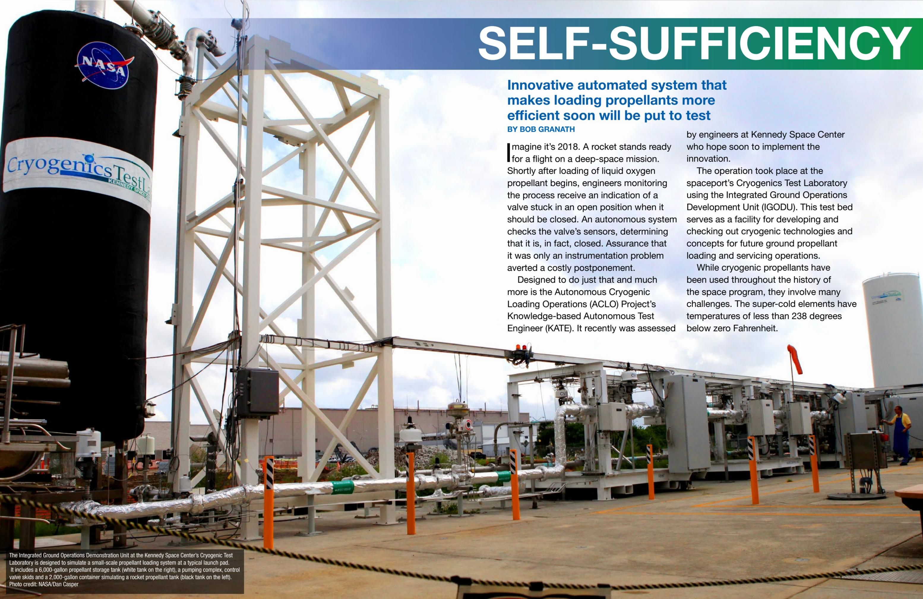
The Integrated Ground Operations Demonstration Unit at the Kennedy Space Center's Cryogenic Test Laboratory is designed to simulate a small-scale propellant loading system at a typical launch pad. It includes a 6,000-gallon propellant storage tank (white tank on the right), a pumping complex, control valve skids and a 2,000-gallon container simulating a rocket propellant tank (black tank on the left). Photo credit: NASA/Dan Casper
