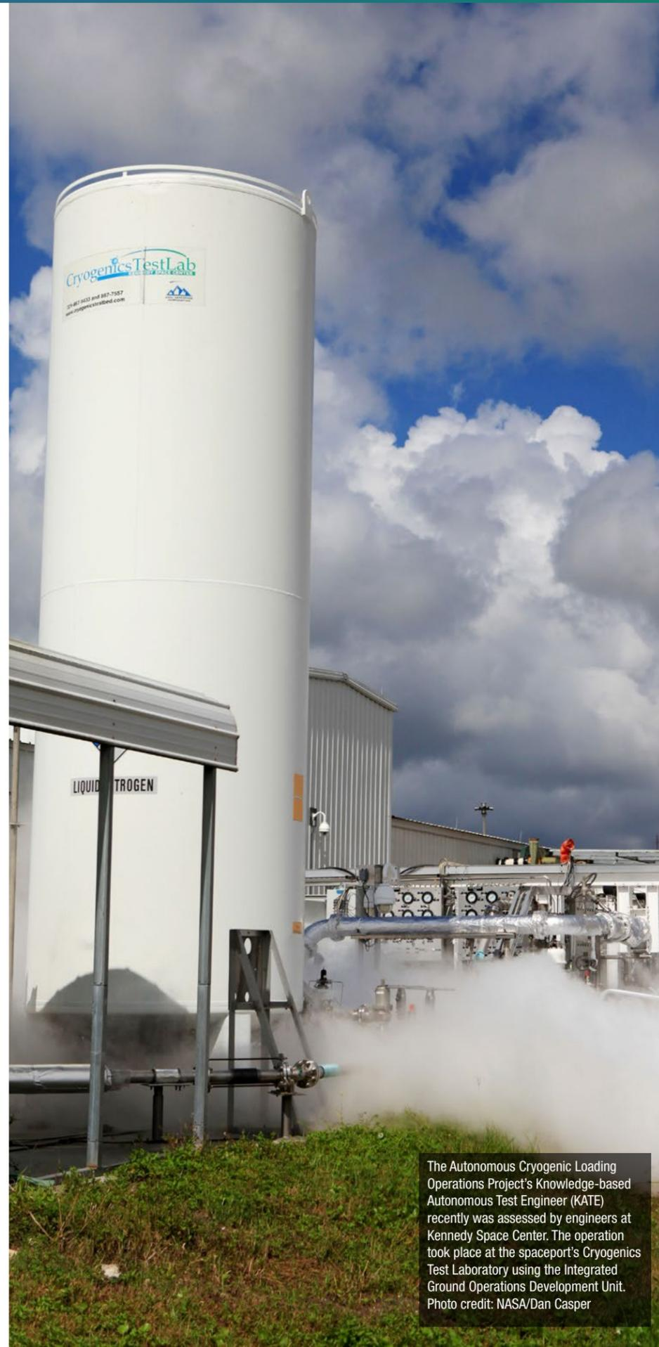
The Autonomous Cryogenic Loading Operations Project's Knowledge-based Autonomous Test Engineer (KATE) recently was assessed by engineers at Kennedy Space Center. The operation took place at the spaceport's Cryogenics Test Laboratory using the Integrated Ground Operations Development Unit. Photo credit: NASA/Dan Casper
