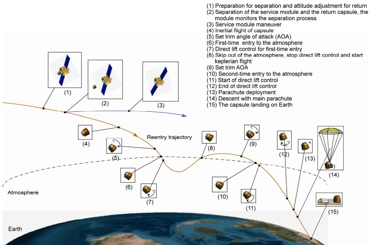
Figure 4 Reentry flight process of reentry capsule.
