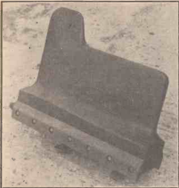
The secret of V-2's perfect stability at take-off was in the four gyro-synchronised vanes, made from graphite, which worked in the jet stream.
