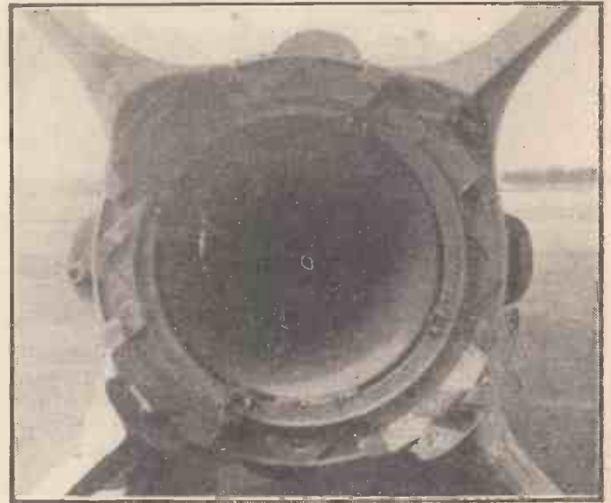
The nozzle end. At the root ends of the four fins are the plates which hold the graphite vanes. Shafts from these extend into the fins and link up with the airstream vanes so that both sets of controllers work in tune with the controlling gyroscopes.
