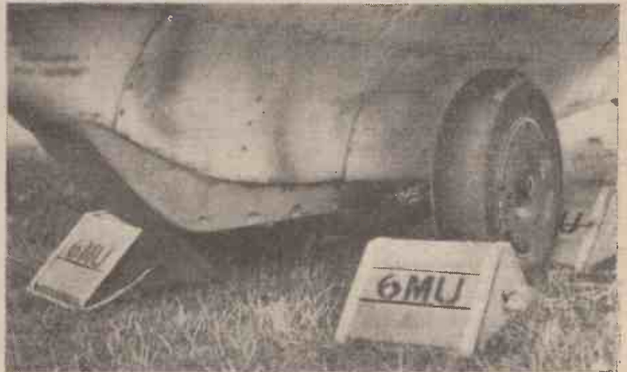
A close-up of the retracted landing-skid and jettisonable take-off chassis of the Messerschmitt 163B.
