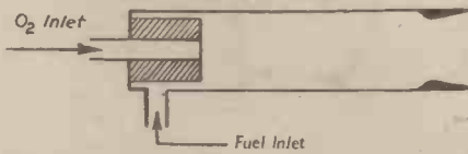
Fig. 16.—Principle of the concentric-feed rocket motor.
