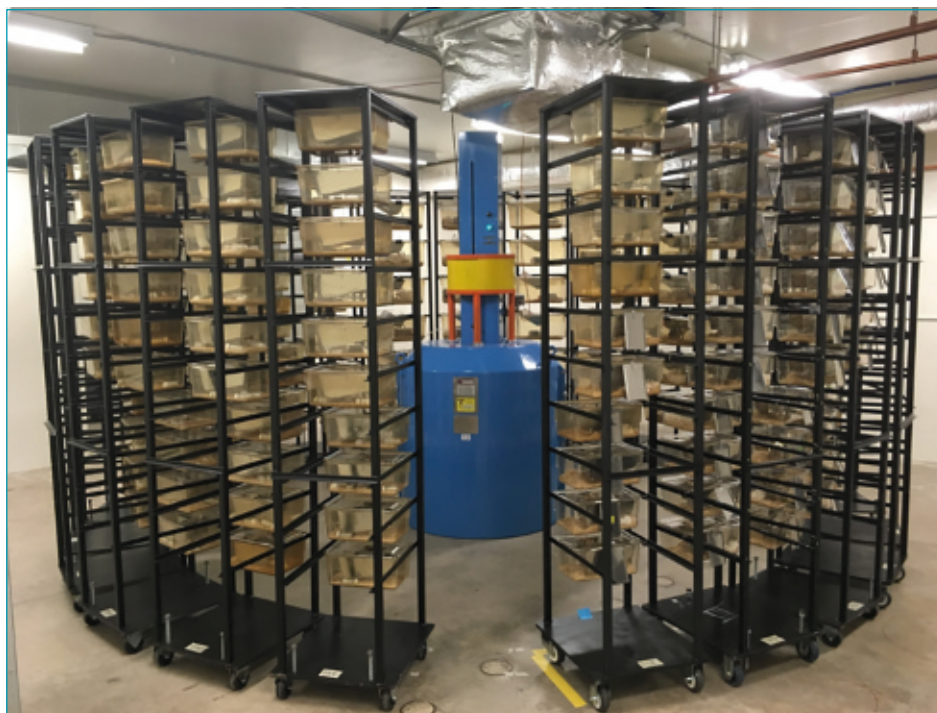
Figure 2. The neutron irradiation facility at CSU. Shown are the annular arrangement of rodent cages around the lead-shielded ^{252}\text{Cf} source that can be lowered and raised for maintenance and animal husbandry procedures. The arrangement of the cages can be modified to accommodate a variety of samples and configurations, and depending on the actual distance from the source, dose rates can be adjusted accordingly.
