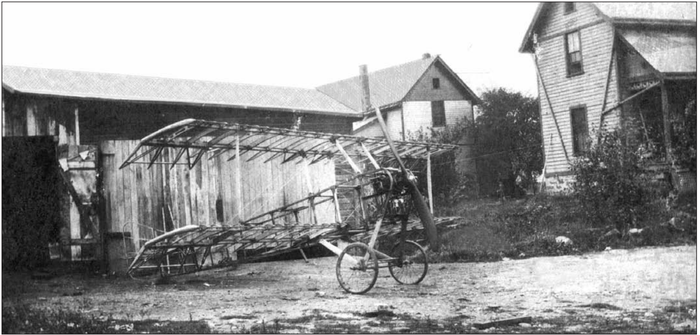
Figure 6. Rebuilt as a biplane, this is the Bleriot frame before it was covered. The photograph was taken behind the Hungerford house at right.
