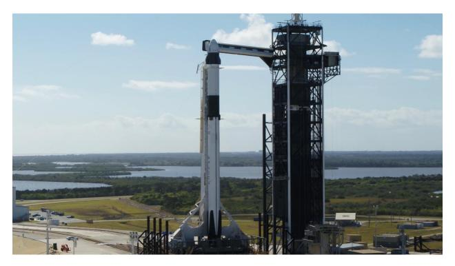
Falcon 9 is a two-stage rocket designed and manufactured by SpaceX for the reliable and safe transport of satellites and the Dragon spacecraft into orbit. Falcon 9 is the first orbital class rocket capable of reflight.
