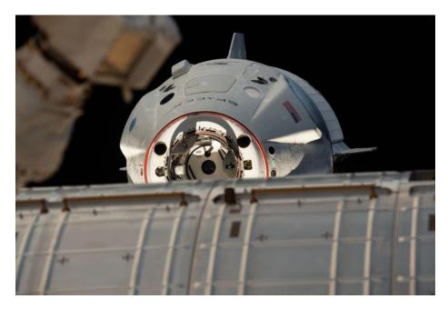
Dragon is composed of two main elements: the capsule, which is designed to carry crew and critical, pressurized cargo, and the trunk, which is an unpressurized service module. The capsule is subdivided into the pressurized section, the service section and the nose cone, which is opened once on orbit and stowed prior to re-entry.
