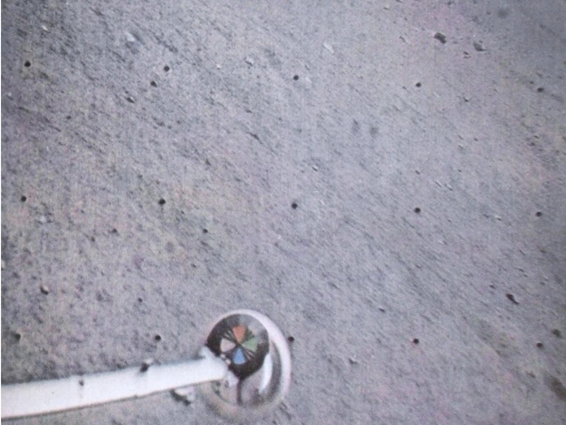
Fig. 11. A photometric target at the tip of omni-directional antenna B provides the only color in this view of the gray lunar landscape as seen by Surveyor I's camera.
