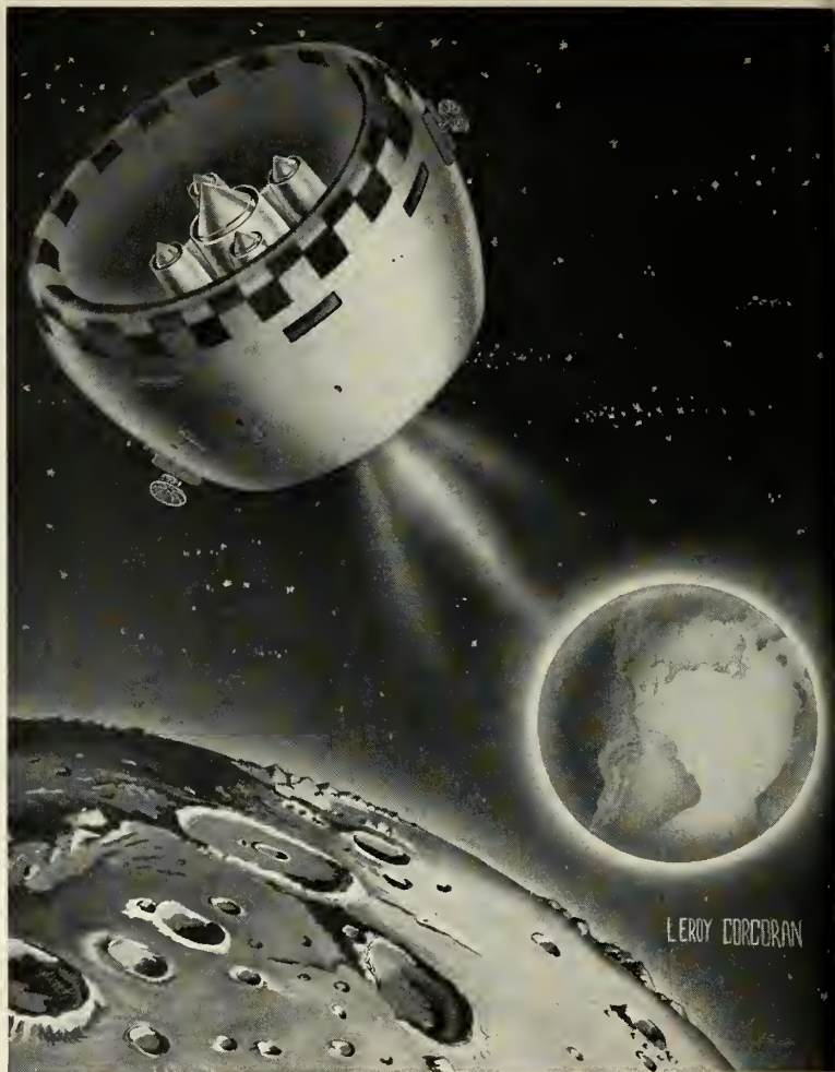
A VIEW of Col. Davis' "conceptual design" as it might appear in flight past the moon. It is operating on its ion propulsion system, having first reached orbital velocity by means of turbo-jets and ramjets.
