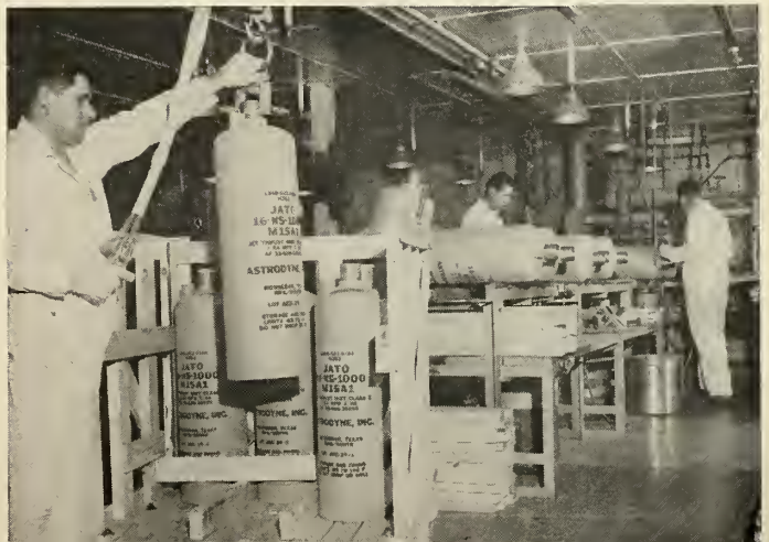
Finished JATO's are loaded nine to a case for shipment to Air Force bases. A protective cap covers each nozzle and igniters are loaded separately in protective tubes inside the crate. Wooden crates are manufactured by a sub-contractor in McGregor, and are used to transport new JATO cases from a second sub-contractor to the plant.
