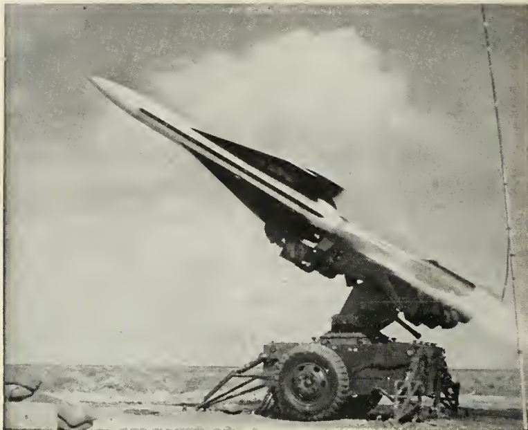
ARMY'S HAWK MISSILE is launched from mobile platform by fast-moving land forces. Raytheon engineers working on prime contract developed the design that makes possible missile's extremely low-altitude capabilities.
