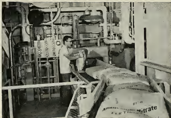
Fertilizer grade ammonium nitrate—used as oxidizer—arrives from line storage building by conveyor. Here bags are being opened for preliminary break-up of large lumps. Material will travel upstairs by skip hoist for start of crushing, drying, and grinding operations. Beyond this point, nitrate is processed by remote control in automatic equipment.
