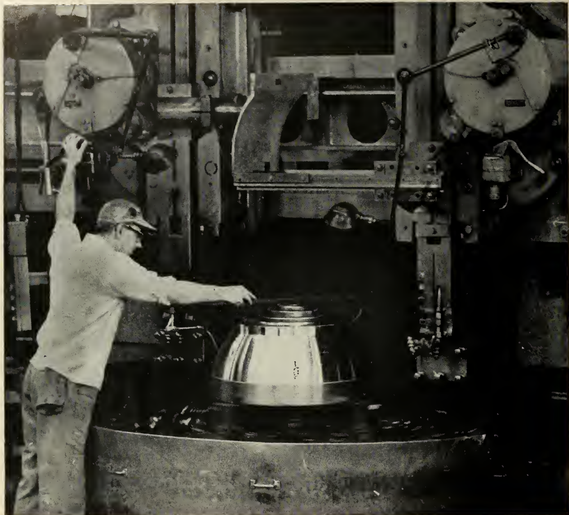
Contour machining of an aft dome for a U.S. Army missile.
