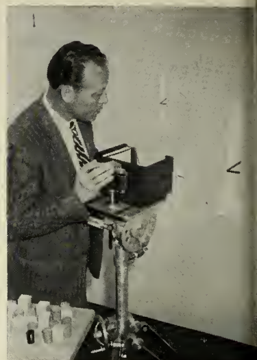
"SHOOTING" RED AND WHITE missile replicas with "haze" box attached to camera, as demonstrated by Raife Tarkington of Kodak Research Laboratories. The box arrangement enables simulation of atmospheric haze on the film.
