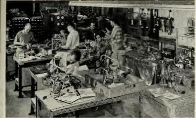
WORKMEN AT ROCKETDYNE Neosho's production plant assemble complete vernier engine systems. Engines are given a routine production check before packaging. Sample hot firings of this production power package are made regularly.
