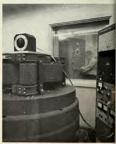
VIBRATION EQUIPMENT is mounted on lead mass for testing a gyroscope. An M-H test engineer views the completed setup through a thick-glass, triple-pane window.
