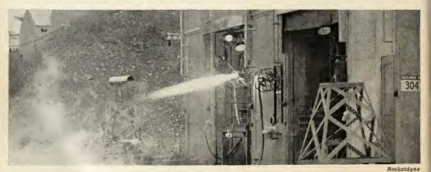
VERNIER ENGINE is subjected to long duration hot fire check. Television and movie cameras film the operation. Additional component test cell areas are in background.
