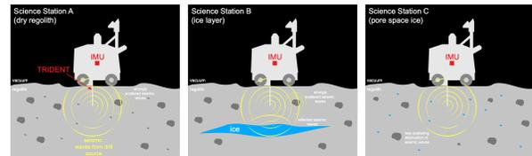
Figure 1. As the VIPER mission traverses across a PSR, differing ice content and expression in the shallow subsurface will result in changes to the response of the ground (e.g., changes in seismic velocity and attenuation) to a vibrating/percussive drill source. We seek to quantify how detectable these signals will be to the rover's IMU.
