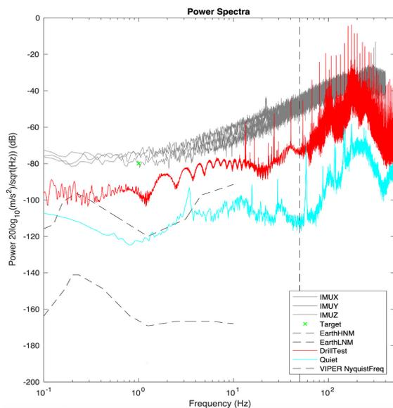
Figure 3. The relationship of background seismic signal to drilling at the Long Valley experiment location (cyan) and the response during the percussive drilling (red, solid) compared to the idealized expected seismic performance of an IMU with performance comparable to the VIPER IMU (grey). The dashed lines are the high and low noise seismic models of the Earth (black) and Mars (red). Drill resonances below the Nyquist frequency of the IMU are present between 10-50 Hz.
