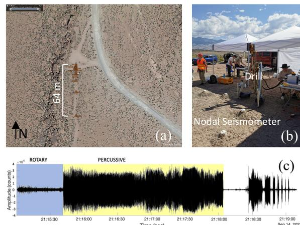
Figure 2. (a) Bishop Tuff field site (37.43°N, -118.42° E, elev. 1341.0 m); (b) field experiment setup; (c) An example of seismic waveforms from the rotary and percussive mode of a TRIDENT-analog instrument
